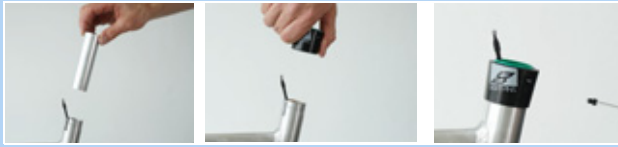
Figure 156: Fitting the slide bushing and outer sleeve
