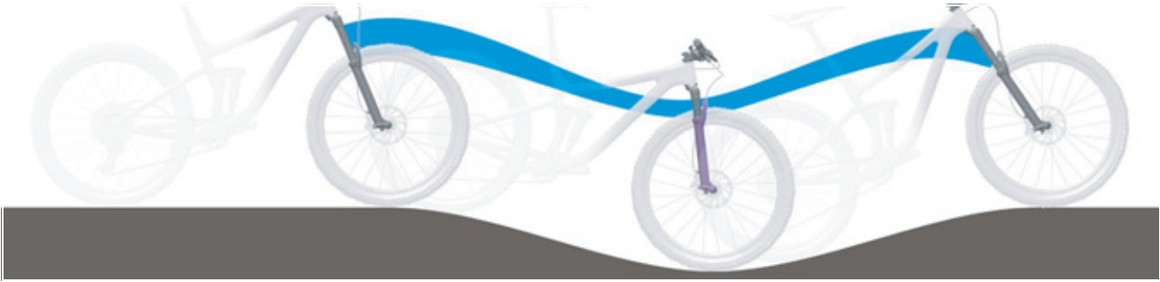
Figure 198: Excessively soft suspension in the suspension fork on hilly terrain
