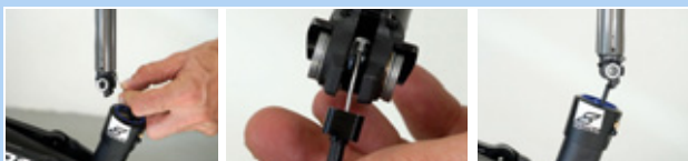
Figure 190: Attaching and pushing in the seat post
