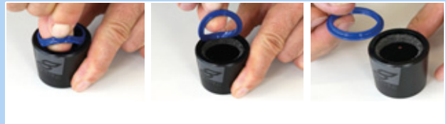
Figure 142: Removing the wiper
