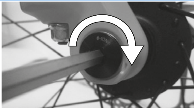
Figure 42: Tighten the axle in the direction of the arrow
