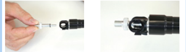
Figure 149: Screwing the valve adapter in
