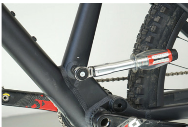
Figure 63: Tightening the seat post axle
