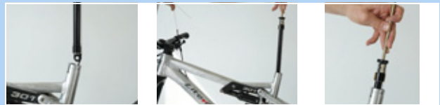
Figure 160: Fastening the cartridge valve lid
