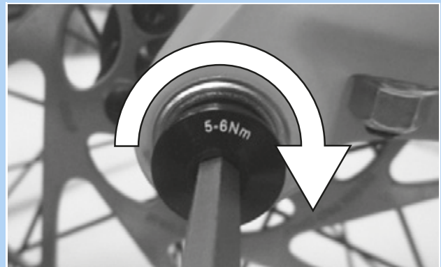
Figure 44: Tightening the securing screw
