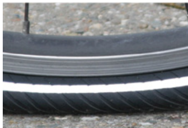
Illustration 82 : Pression largement insuffisante
