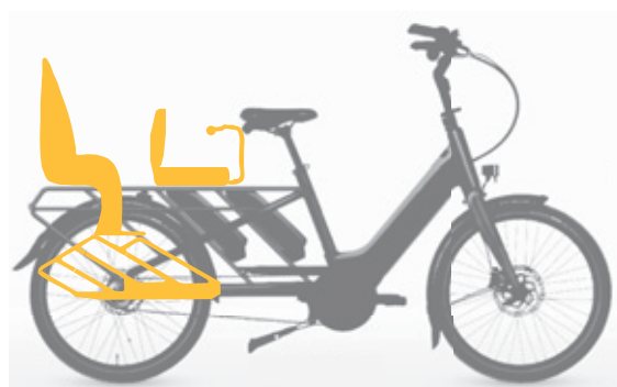
Figure 22: A child seat at the rear and a saddle seat with sideblades in front, suitable for one young child (1–6 years old, 9–22 kg) and an older child (6–10 years old, 18–38 kg)
