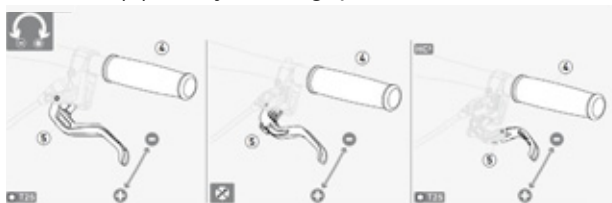
Figure 19: Setting the grip distance on a Magura disc brake lever
