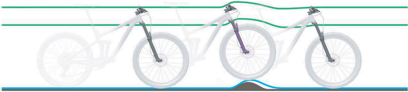
Figure 195: Excessively hard damping in the suspension fork on bumps
