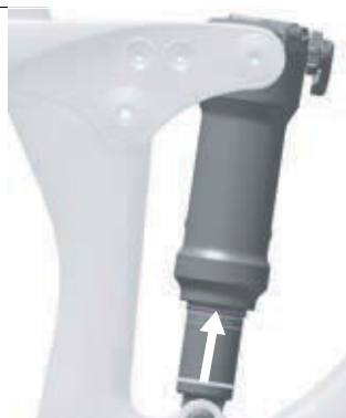
Figure 116: Moving the O-ring on the rear frame damper
