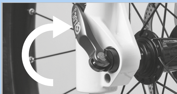
Figure 71: Closing the quick release
