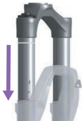
Figure 108: Moving the O-ring on the suspension fork
