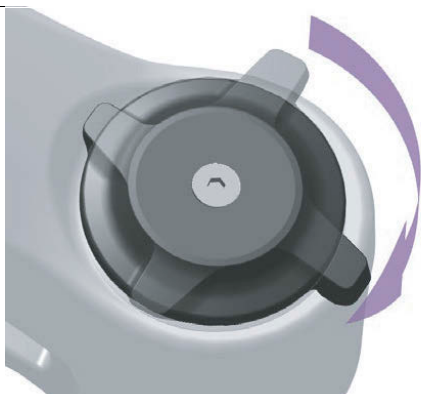
Figure 194: Changing compression adjuster to a harder setting
