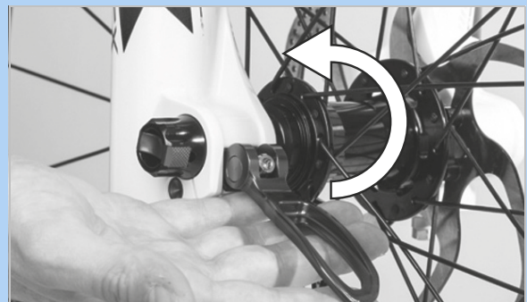
Figure 65: Pressing the quick release lever in the direction of the arrow
