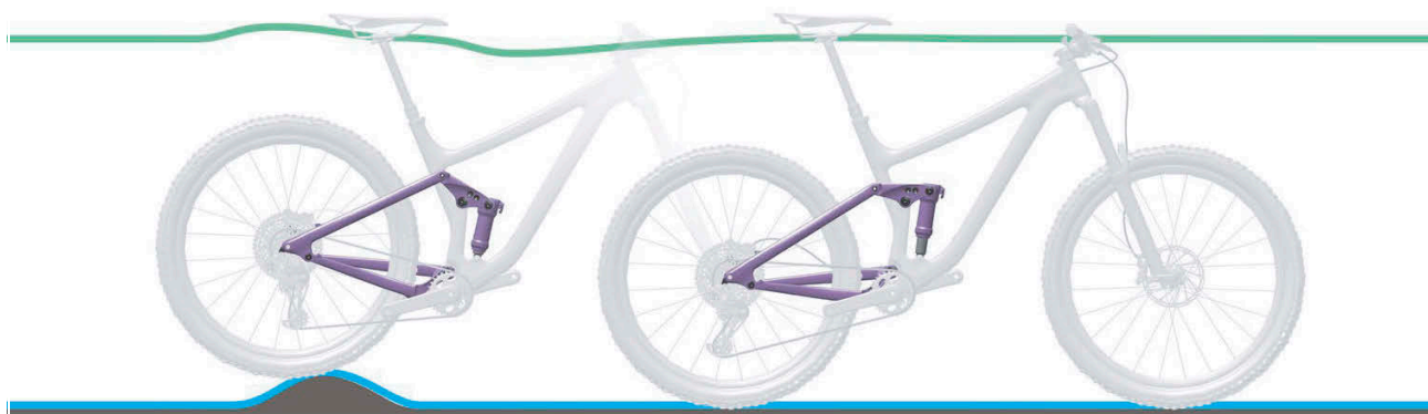
Figure 121: Optimum rear frame damper ride performance over bumps
