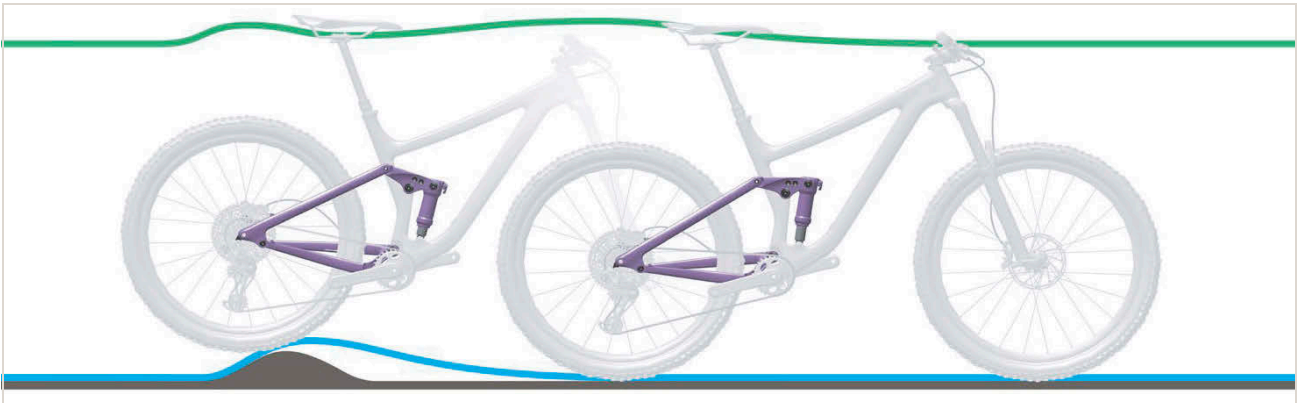
Figure 203: Excessively hard damping in the rear frame damper on bumps
