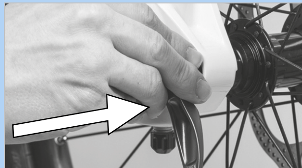
Figure 69: Inserting the quick release in the direction of the arrow
