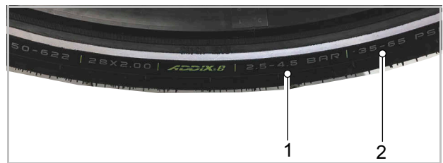
Figure 165: Tyre pressure specification in bar (1) and psi (2)
