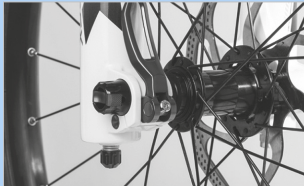
Figure 185: Adjusting the quick release clamping force
