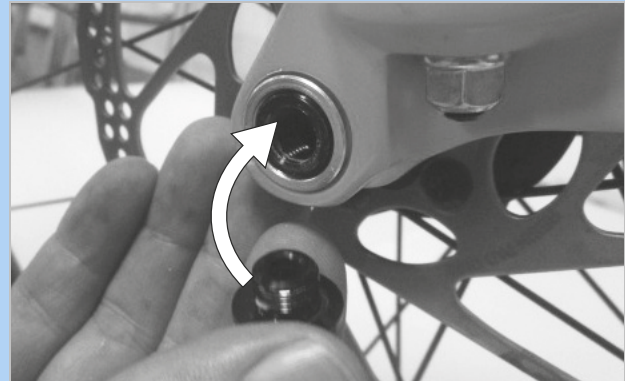
Figure 60: Inserting the securing screw
