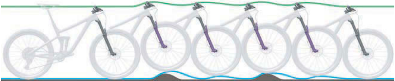
Figure 189: Suspension fork rebounding too quickly
