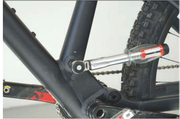
Figure 77: Tightening the seat post axle
