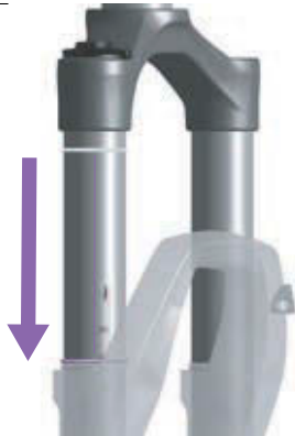
Figure 111: Moving the O-ring on the suspension fork
