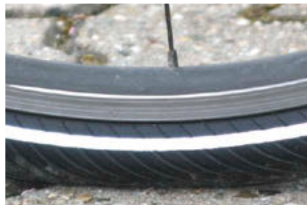
Figure 99: Correct tyre pressure. The tyre is barely deformed under the load of the body weight
