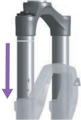
Figure 102: Moving the O-ring on the suspension fork
