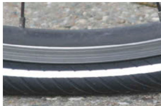
Figure 100: Much too little tyre pressure
