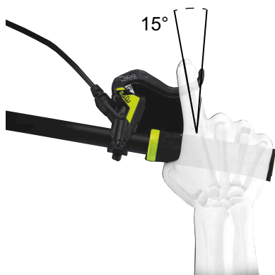
Figure 95: Brake handle position
