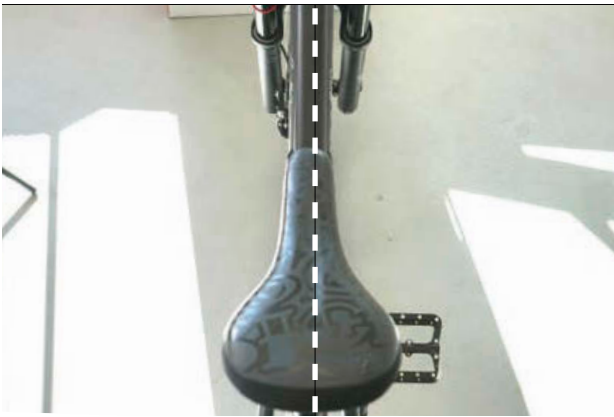
Figure 76: Positioning the saddle in direction of travel
