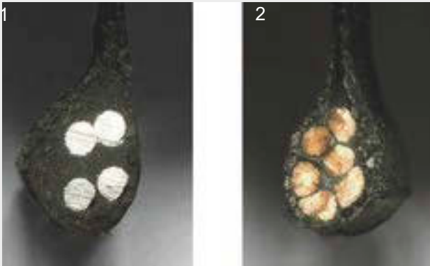
Figure 19: Steel bead core (1) and Kevlar bead core (2)
