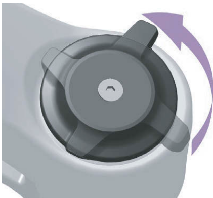
Figure 196: Adjust the compression adjuster so that it is softer
