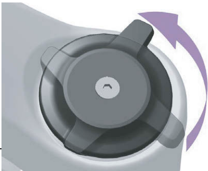
Figure 158: Changing compression adjuster to a softer setting
