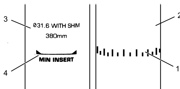
Figure 80: Detailed view of the seat post – examples of the minimum insertion depth marking
