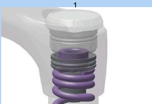
Figure 105: Screwing and unscrewing the preload adjustment ring
