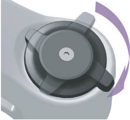
Figure 157: Changing compression adjuster to a harder setting
