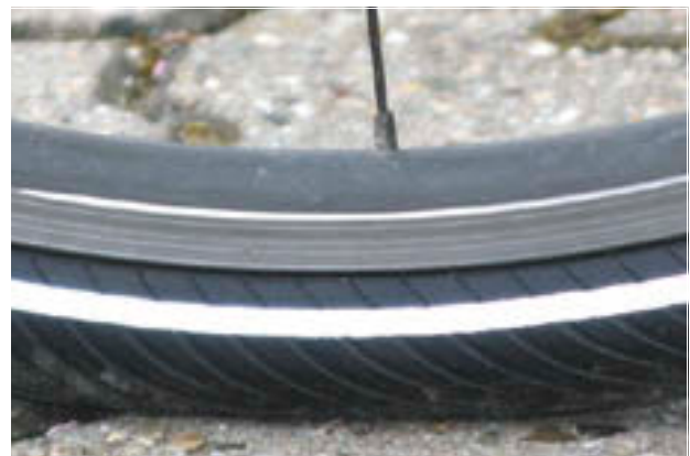
Figure 93: Correct tyre pressure. The tyre is barely deformed under the load of the body weight
