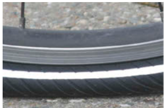
Figure 94: Much too little tyre pressure
