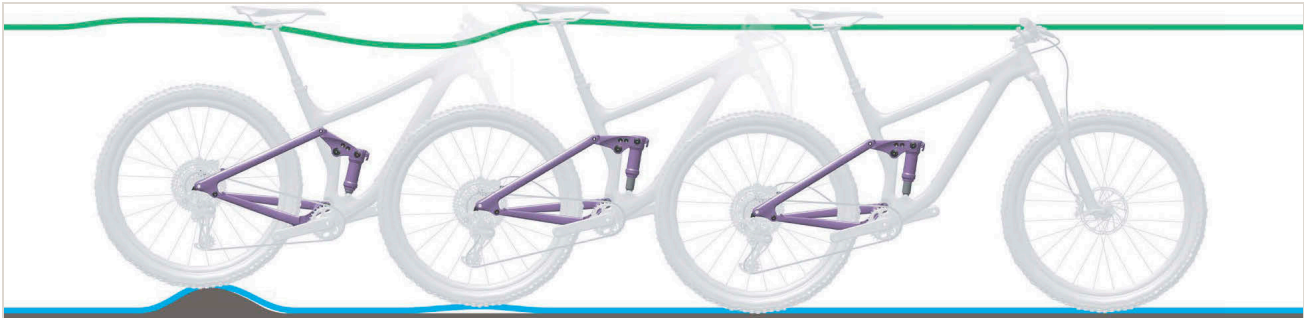
Figure 197: Rear frame damper rebounding too quickly
