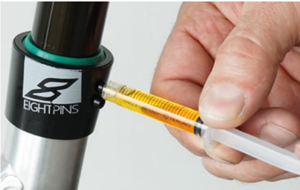
Figure 144: Lubricating the seat post tube
