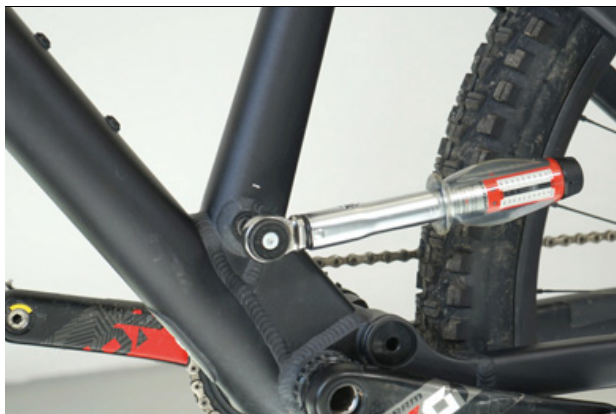
Figure 66: Tightening the seat post axle
