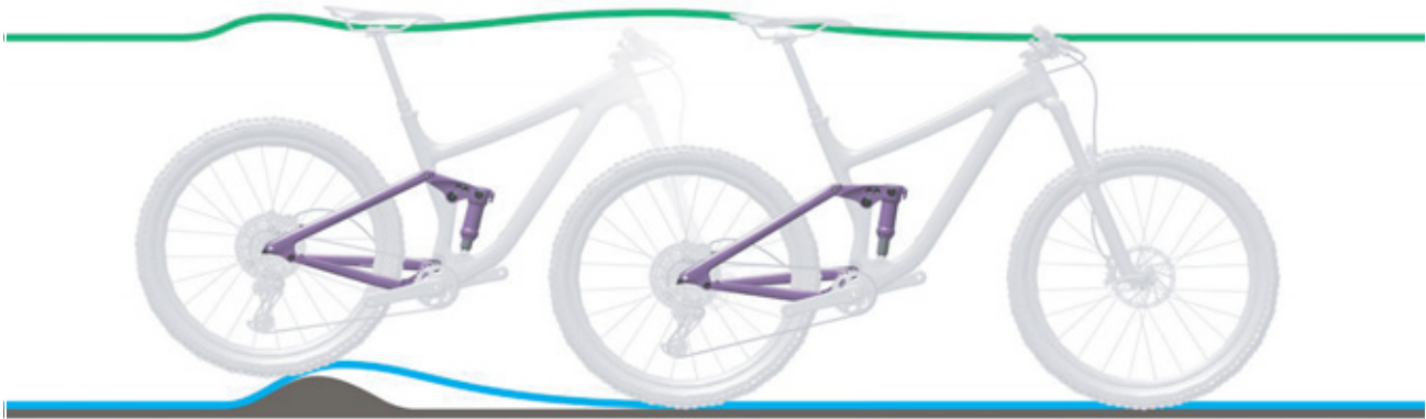
Figure 237: Excessively hard damping in the rear frame damper on bumps
