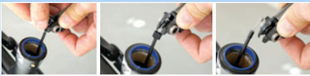
Figure 200: Removing the Bowden cable
