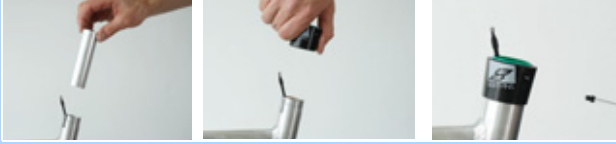
Figure 216: Fitting the slide bushing and outer sleeve
