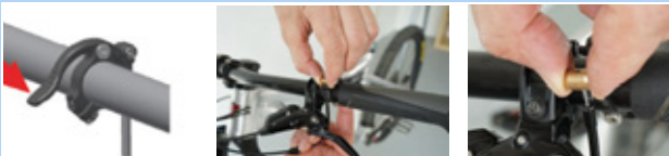
Figure 161: Removing the cartridge
