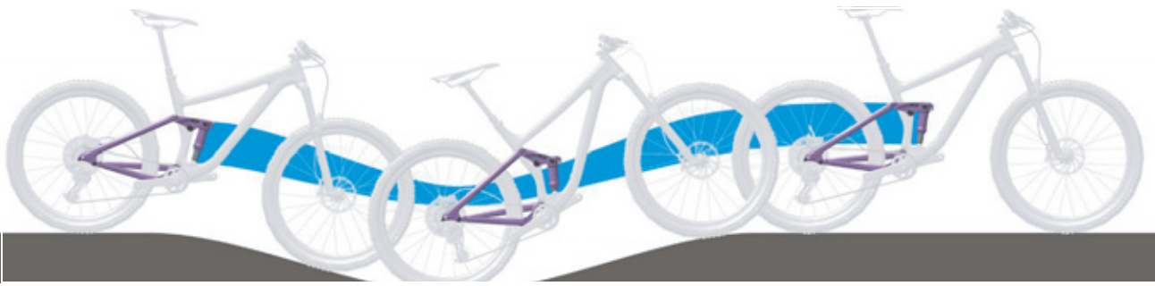
Figure 235: Excessively soft suspension in the rear frame damper on hilly terrain
