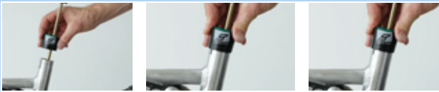
Figure 191: Attaching the outer sleeve
