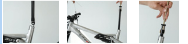
Figure 187: Fastening the cartridge valve lid
