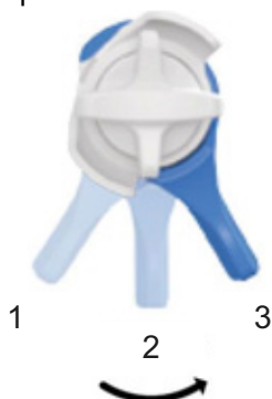
Figure 89: Adjustment of the 3-way lever from closed (1) to intermediate (2) to open (3)
