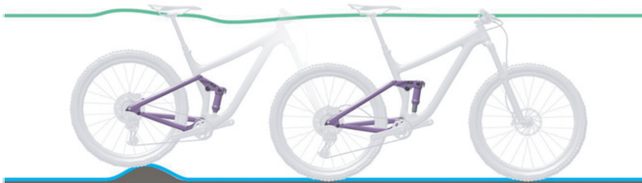
Figure 133: Optimum rear frame damper ride performance over bumps
