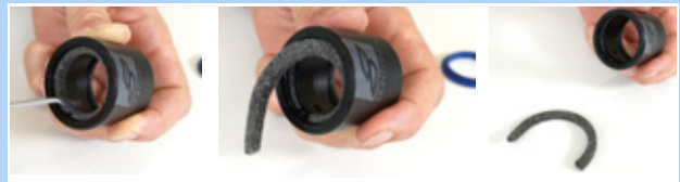
Figure 170: Removing the felt ring
