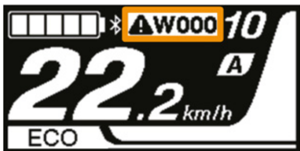
Figure 62: Example: Warning W000
