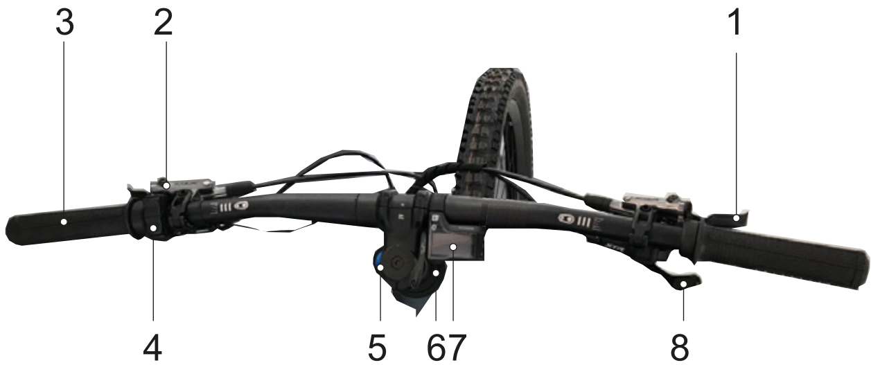
Figure 42: Detailed view of handlebars with SHIMANO SC-E800 on-board computer, used as example
