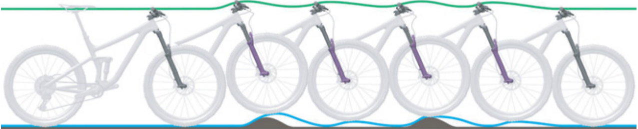
Figure 221: Suspension fork rebounding too quickly
