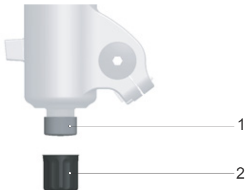
Figure 222: FOX rebound screw (1) under fork cap (2)
